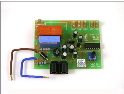
Automatic Hand Dryer Control Unit with IR sensor
